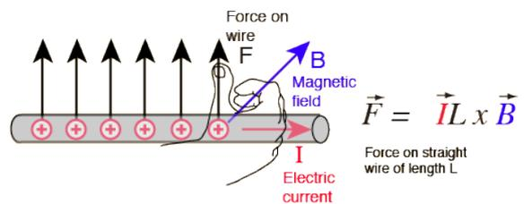
$$\vec{F} = q(\vec{v} \times \vec{B}) = q \left( \frac{\vec{l}}{t} \times \vec{B} \right) = \frac{q}{t} (\vec{l} \times \vec{B}) = I (\vec{l} \times \vec{B})$$
